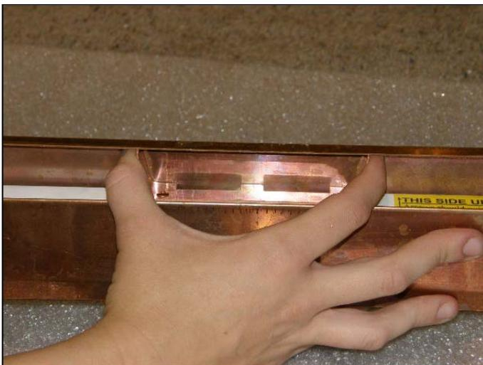
When replacing it; once it is in, be sure it is square to the Water Distribution Unit, then bend the upper tabs up until they push against the top lip of the Water Distribution Unit. Doing this will keep the Baffle firmly in place and allow the water to flow properly.
