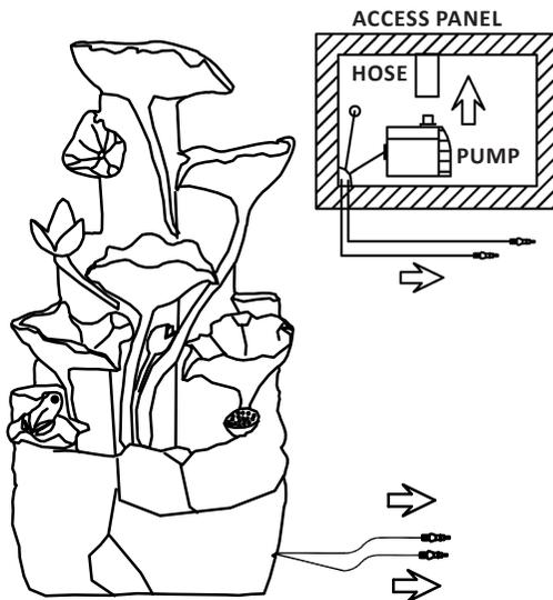
3. Fill the reservoir with water, ensuring the pump will remain completely submerged during operation.
