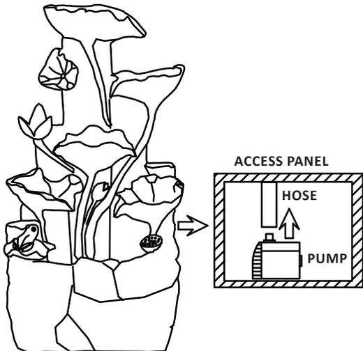
2. Extend the pump and LED light cables through the access panel in the back of the fountain, cables are ready for connection to the solar panel.
