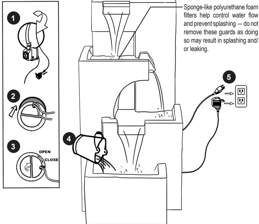
1. From the access panel in the back of the fountain, locate the built-in water tube and light cable. Extend the LED light cable and connect the AC adapter. Connect the pump to the water tube and place the pump inside the fountain.
